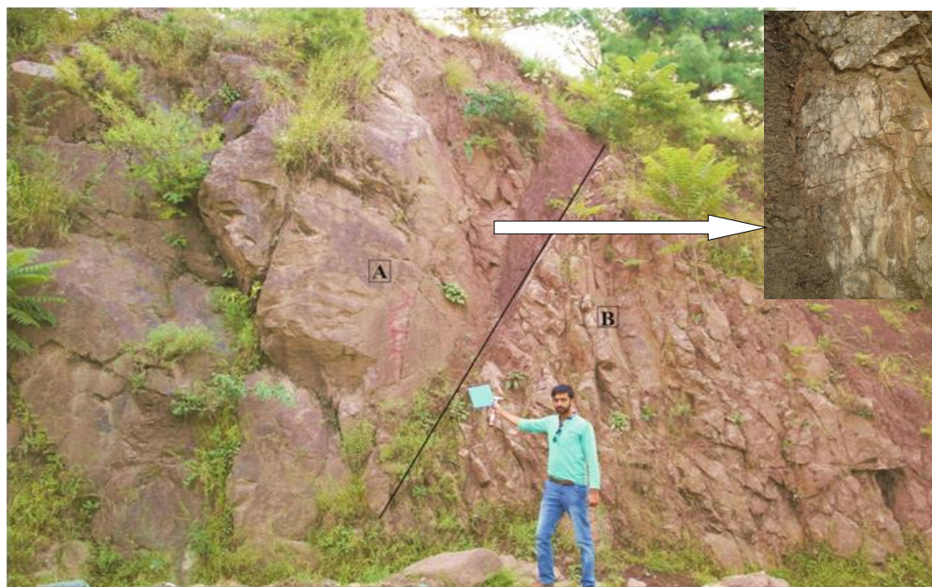
Fig. 10: The Dhirkot Fault marked along Dhirkot Rangla road, where Murree Formation (A) is thrust over Kamlial Formation (B). 3402.571 N 7334.661 E
